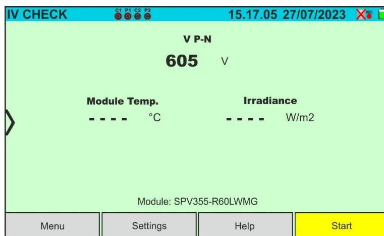
Fig. 73: IVCK test screen with SOLAR03 in synchronous recording on Monofacial modules
