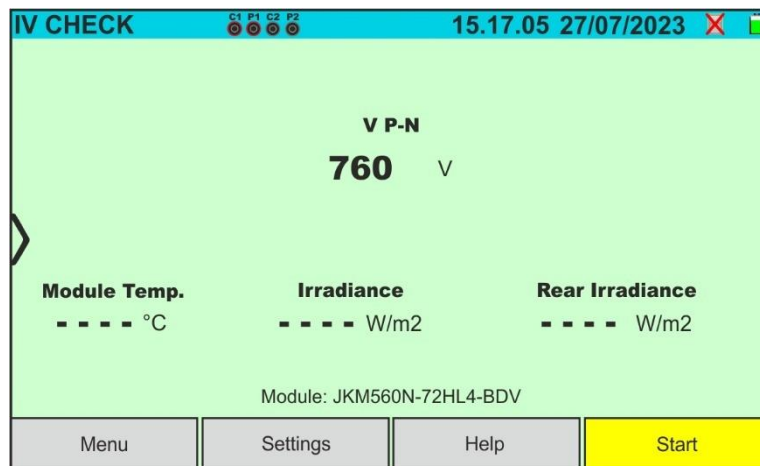
Fig. 58: Initial IVCK test screen without remote unit on Bifacial modules
