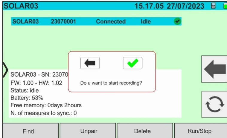
Fig. 71: Recording Activation on Remote Unit - Step 1
