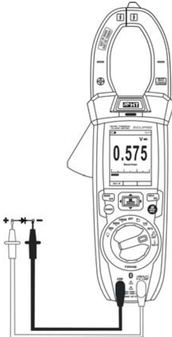
Fig. 28: Use of the instrument for diode test
