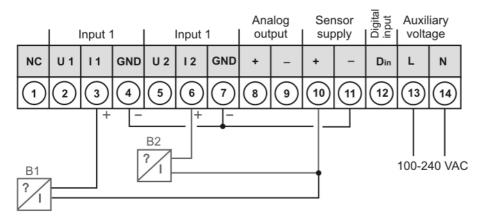
Co-channel measurement with voltage signals, supply 10-40 VDC:
