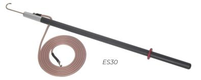
The ES30, ES50 and ES100 earthing sticks are designed for earthing the high voltage connection after ac testing in accordance with EN50191. The earthing sticks consist of a hooked earth connection mounted on an insulated handle with a 5m earth lead. The earth lead insulation is clear silicone allowing the conductor to be easily inspected, and is terminated in an M6 hooked crimp.
