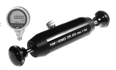
Our Hand Pump/Volume Regulator 8135 is a very handy tool for the generation and adjustment of pneumatic pressures. This unit can generate pressures up to approx. 5 bar. The plastic casing of the pump is designed to assure maximum grip. This material also prevents heat transfer by e.g. hand warmth.
