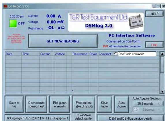
Connecting the DSM600 to a PC running the optional DSMlog software adds data capture and reporting functions to the unit, allowing test results to be exported directly to Excel or saved to a file. All results are time stamped, and a comment may be added to each test. Data capture can be controlled from the PC, and the resistance of a test object can be monitored over a period of time.
