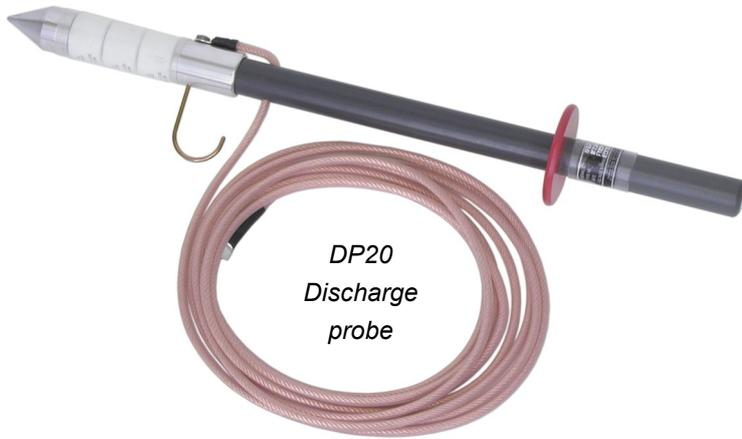
The DP20 and DP40 discharge probes are designed for discharging high voltage cables after testing. The probes are supplied as standard accessories for the T&R PT18-10 and PT30-10 cable test sets, and are also available separately.
