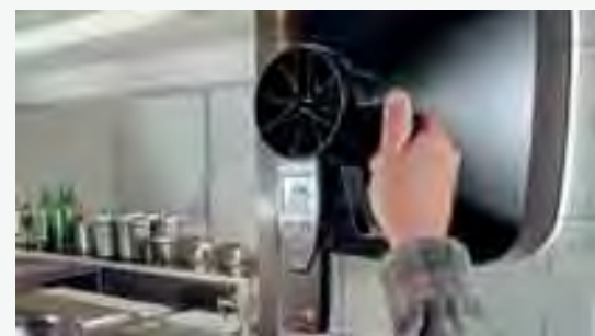
Monitors outgoing air in an on-wall ventilator
